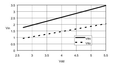
Figure 13 Typical Schmitt Trigger Input Voltage Thresholds vs. V<sub>DD</sub>
