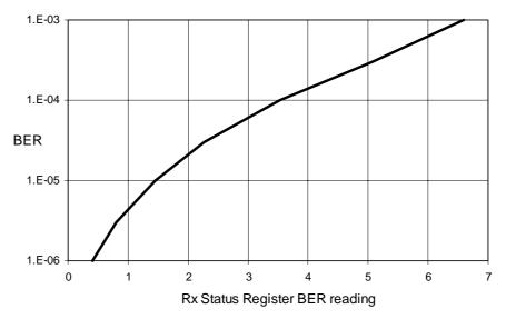
Figure 11 Typical Rx BER vs. Average Status Register BER Reading (b2-0)
