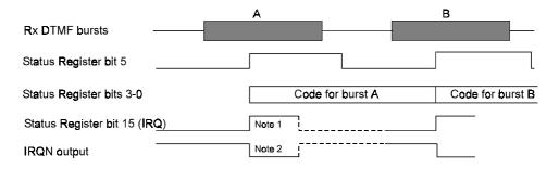
Notes: 1. IRQ will go high only if the IRQ Mask bit b0 in the General Control Register is set. The IRQ bit is cleared by a read of the Status Register.
