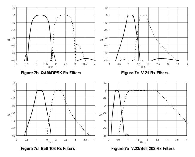
The signal level at the output of the Receive Modem Filter and Equaliser is measured in the Modem Energy Detector block, compared to a threshold value, and the result controls bit 10 of the Status Register.
