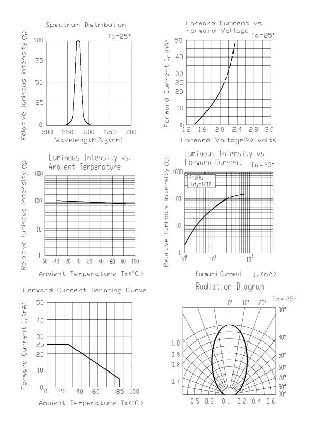
Everlight Electronics Co., Ltd. Device No. : DSE-111-G04 http://www.everlight.com Prepared date: 08-02-04 Rev.1.0 Page: 4 of 9 Prepared by: Kenny Wang
