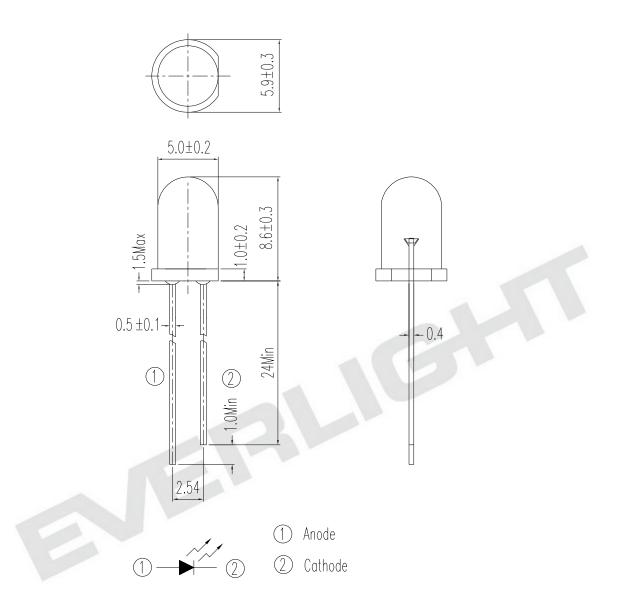
Note: Tolerances unless dimensions ±0.25mm
