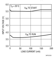
Minimum Input Voltage,  $V_{OUT} = 5V$
