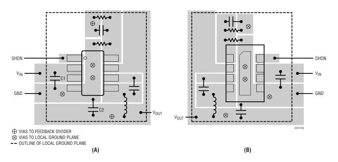
Figure 5. A Good PCB Layout Ensures Proper, Low EMI Operation
