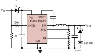
Figure 4. Diode D1 Prevents a Shorted Input from Discharging a Backup Battery Tied to the Output; It Also Protects the Circuit from a Reversed Input. The LT3470 Runs Only When the Input is Present Hot-Plugging Safely
