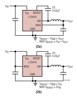
Figure 2. Two Circuits for Generating the Boost Voltage
