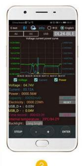
upper right corner shows the model currently online. DL24-BLE The bluetooth icon in the upper left corner turns blue, indicating that the measurement is in online communication.
