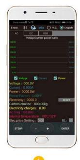
When the USB tester is powered on, the Bluetooth indicator is flashing, turn on the pop up the menu for selecting E-test App softare icon , and the USB tester model, DL24-BLE, allow Bluetooth to turn on.
