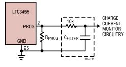
Figure 11. Monitoring Average Charge Current
