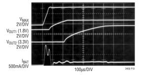
Figure 10. In-Rush Current at Startup
