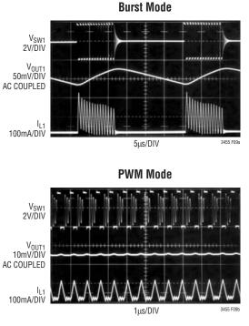
Figure 9. Burst Mode and PWM Mode Waveforms
