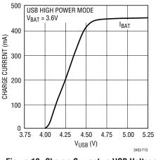
Figure 13. Charge Current vs USB Voltage
