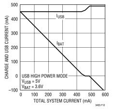
Figure 12. Charge Current vs Total System Current
