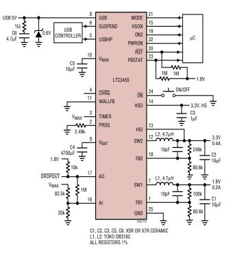
Figure 16. Standalone USB Power Supply with Temporary Backup Power
