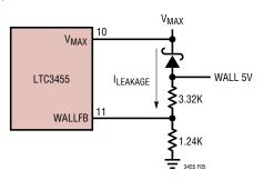
Figure 5. Schottky Leakage Current Path
