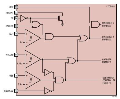
Figure 3. Turn-On Logic Diagram for LTC3455
