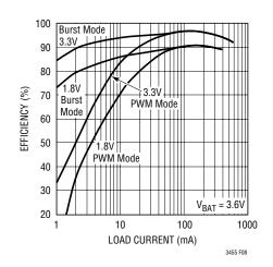
Figure 8. PWM and Burst Mode Efficiency
