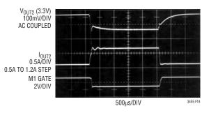
Figure 18. Load Current Step (0.5A to 1.2A) for 3.3V Output
