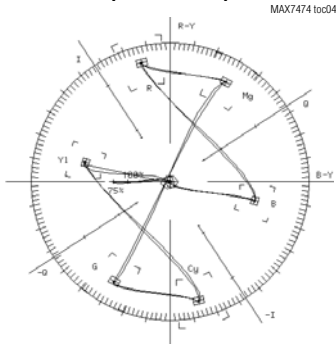
75% COLOR BAR VECTOR DIAGRAM (300m CABLE)
