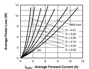
Fig. 6 - Forward Power Loss Characteristics
