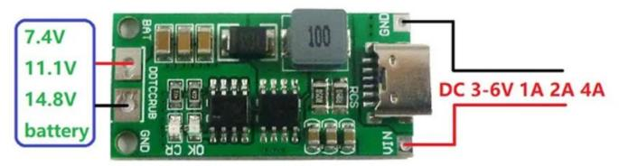
Note: For the 2A/4A version, please provide a power supply greater than 2A/4A and good soldering.
