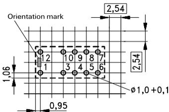
Note: Hole for pin 6 and 7 only for latching with 2 coils
