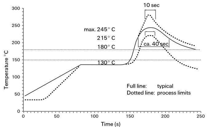
Infrared Soldering: Temperature/Time Profile (Lead Temperature)
