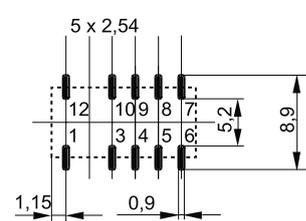
Note: Solder pad for pin 6 and 7 only for latching with 2 coils
