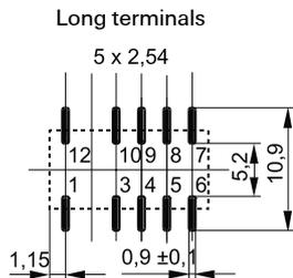
Note: Solder pad for pin 6 and 7 only for latching with 2 coils
