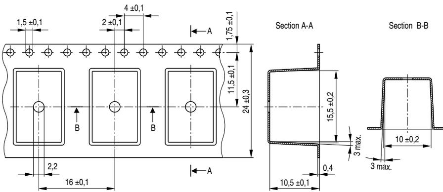
Tape and reel for SMT version with short terminals - 500 relays per reel, 2500 relays per box
