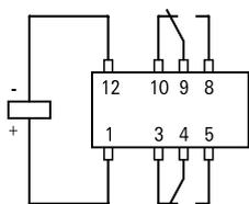
Latching type, 1 coil reset condition
