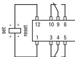
Latching type, 2 coils reset condition
