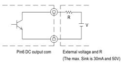
Fig 2.2 Internal circuit of AC OK (Battery Low)
