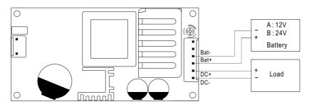
Fig 1.1 Suggested system connection
