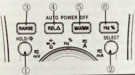
Push once to hold the current reading on the display; push again to continue normal operation.
