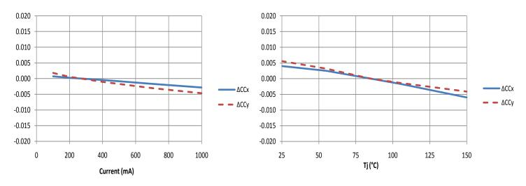
The following graphs represent typical chromaticity vs current and temperature for the XLamp CXA2011 at **5000K** CCT.
