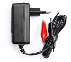
**CL14.4VDC-1.2A** is a plug shape 16-watt lead-acid batteries charger. It supports various types such as flooded, sealed, gel, and VRLA with a nominal voltage of 12 V. The charger supports normal speed in charging mode and next keeps the batteries in standby. It is based on high quality electronic components that allow continuous, long-lasting work in all environmental conditions.
