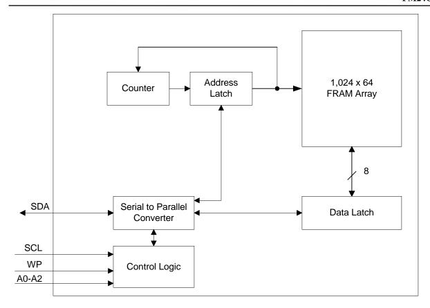
Figure 1. FM24C64 Block Diagram
