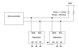
Figure 2. Typical System Configuration
