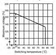
Note: The maximum coil voltage is the maximum value in a varying range of operating power voltages not a continuous voltage
