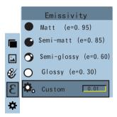
As shown in the figure, press " key to enter the main menu and select " E "(emissivity) option and press " vey to enter the emissivity list.
