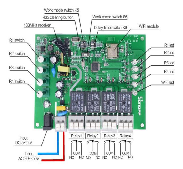
You may choose to power up by 5-24V DC or by 90-250V AC. Each relay without voltage output.
