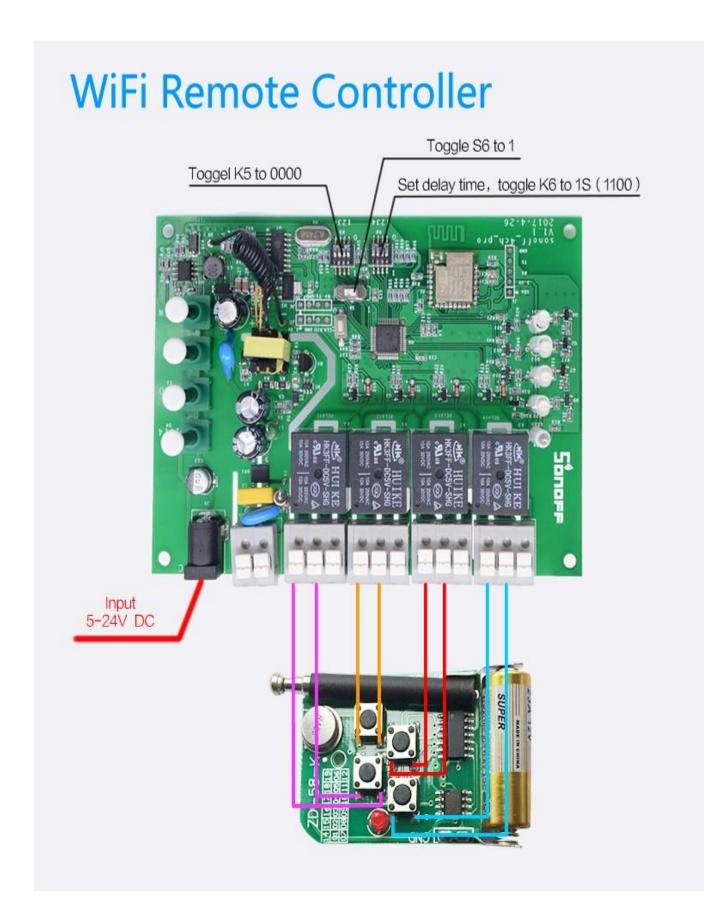
Working Mode Settings RF Remote Settings 1. Power up your device through 90-250v AC(50/60Hz) or 5-24v DC.
