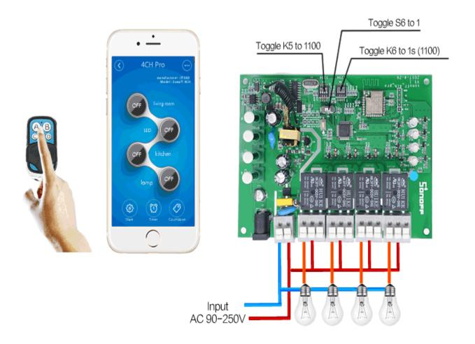
2. In inching mode, you can turn on the connected devices for 1-16s . For example, you can turn on CH1 connected device for 1s, then auto-off.
