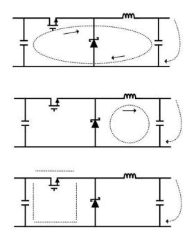
Figure 23. Typical Current Flow in Buck Regulator
