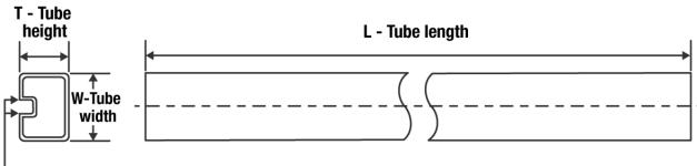
B - Alignment groove width
