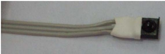
Adopt oblate three-way wire, and connect an infrared receiver to receive an external infrared.
