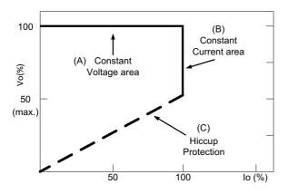
Typical LED power supply I-V curve
