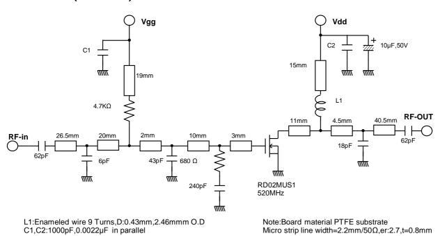
RoHS Compliant, Silicon MOSFET Power Transistor 175MHz,520MHz,2W
