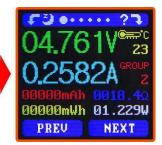
flashing. When the accumulated mAh exceeds 1 mAh, the previous data will be cleared and accumulation will restart.
