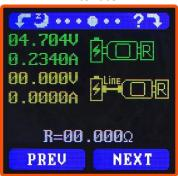
Data Connection Cable Impedance Measurement Interface
